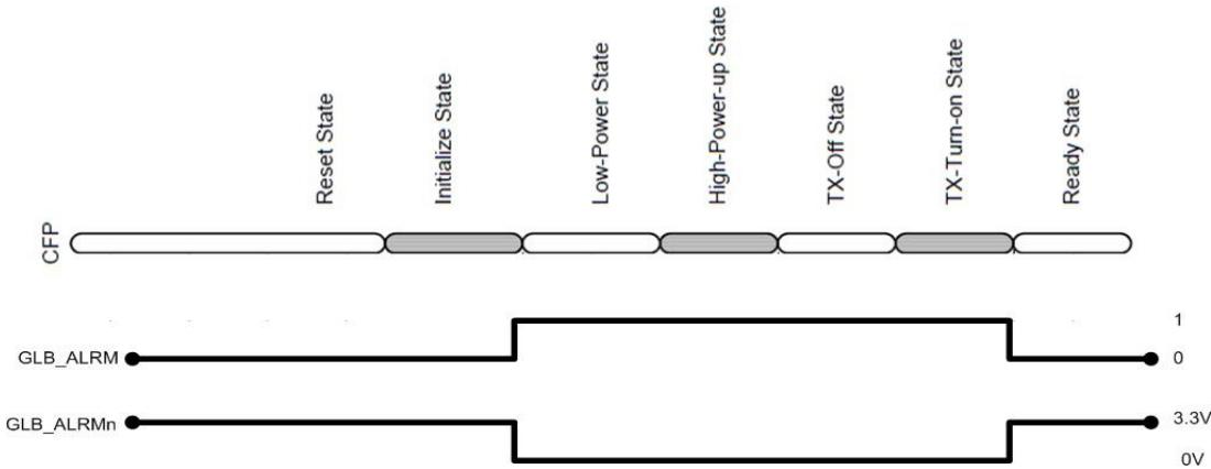
GLB\_ALRM is de-asserted during Reset and Initialize state, it is asserted in Low-Power, High-Power-up, TX-Off and TX-Turn-on states, then de-asserted again when Ready state is reached.
